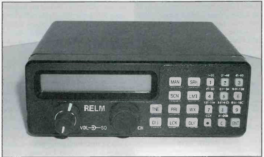
You might find a mobile unit like this works great in your car, but you might also like a smaller unit like this for your base radio. This model from RELM includes tone squelch to reduce interference in high traffic areas.
