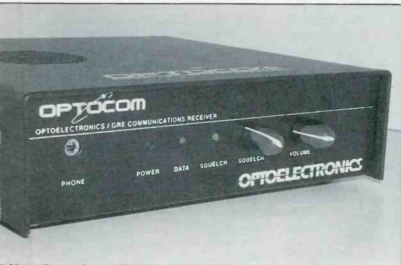
Advanced computer-controlled radios like this new Optocom receiver offer many advanced features, and all the advantages of computer control at a reasonable price since the computer handles most of the hard stuff. This particular unit is quite well-equipped and an excellent choice for getting started with computer-controlled scanning in either a trunked or non-trunked area.
