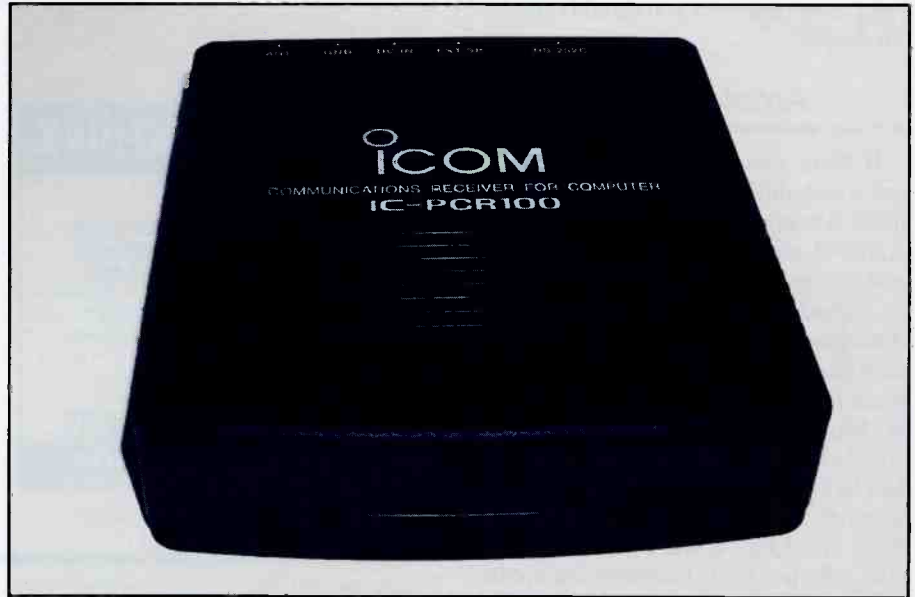
There isn't much to see on the front of this receiver. On the right side, a power light indicates when the unit is in use and that's it for useful information from the receiver itself.
