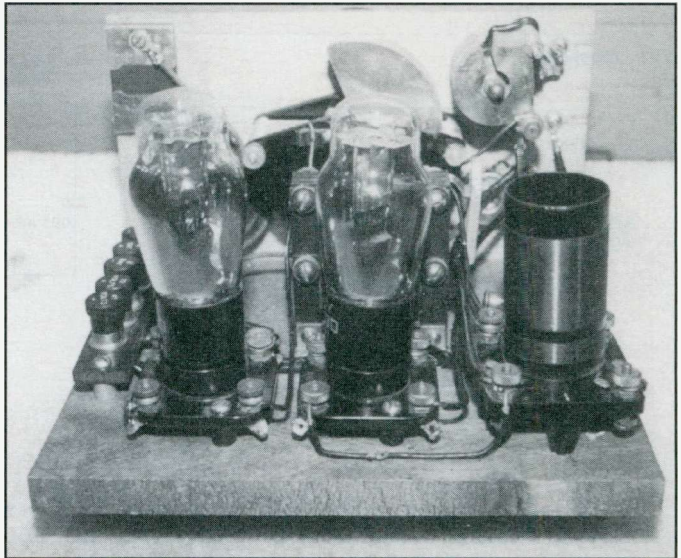
Rear view of receiver. The set was made for four-pin triodes such as the '30 or '99. With a 6-volt "A" supply, 01A or 01AA (100 mA) tubes could probably be used. Type 30s are shown.
