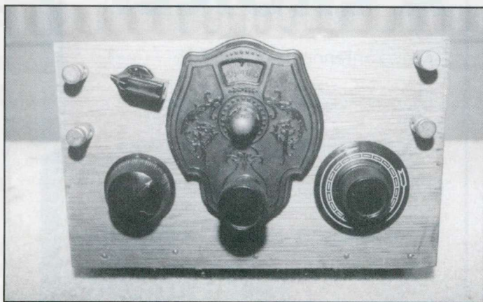
The front-panel view of the new two-tube regenerative receiver. Front panel controls are as follows: upper left, antenna coupling; bottom left, regeneration; center, main tuning dial; and at right, the filament rheostat. Metal binding posts at upper left are for the antenna and ground connections. The headset is connected to the metal binding posts in the upper right side.
