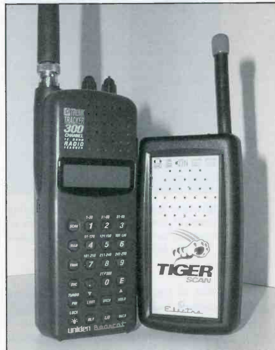
Even handhelds run quite a wide range. On the right, the two-channel, VHF-only Tiger-Scan, and left, the 300-channel BC-235.
